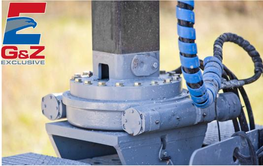
The **AccuSteer** system using hydraulic motor driven slew drives with 320 degree rotation offers unparalleled maneuverability and accuracy, allowing synchronized steering in 90 degree mode in every swing leg position.
