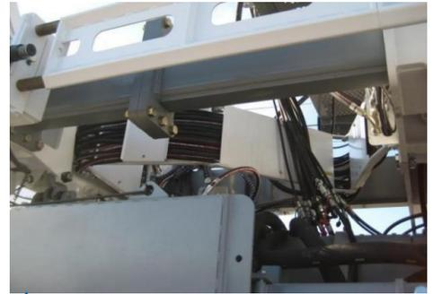
Each side of the the tractor frame is provided with a hose hinge matching the 7ft (2.13m) of telescopic ability of the frame per side.
