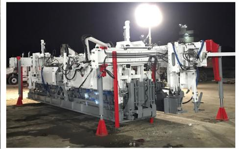
With the selection of the optional DBI Self Loading Jacks, the modular DBI can be self-loaded on a trailer without the use of a crane, saving time and money.
