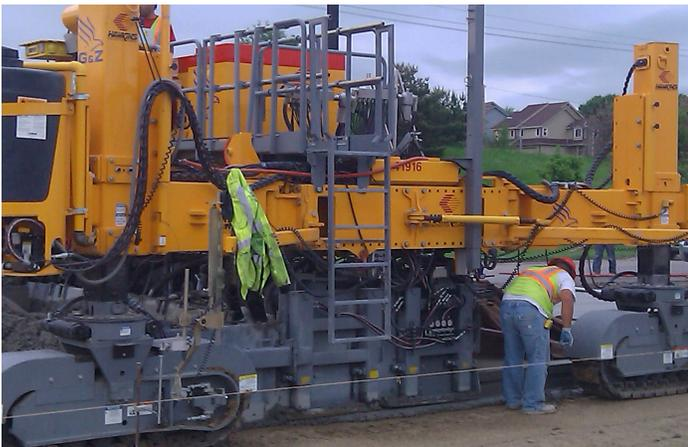
As an option, Guillotine Sideforms with -2 to 18" (-50 to 457mm) of hydraulic adjustment can be supplied split, allowing independent adjustment of the front and rear portions of the sideform. The rear half of the sideform is equipped with hydraulic open / close cylinders which are powerful enough to close against plastic concrete.
