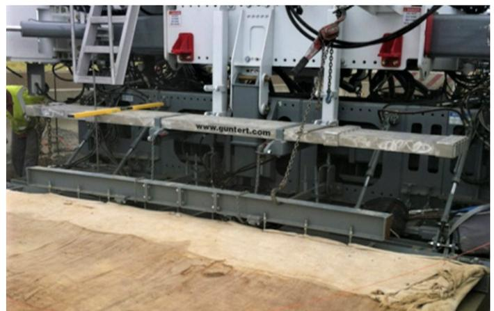
For extra smoothness, the S600 can be fitted with G&Z's optional Trailing Finishing Pan (TFP). The 48 in. (1.2m) wide TFP with fixed edger pans provides a proven method of finishing the pavement surface with fine adjustment, ensuring sharp edges. It also accommodates a wide range of side bar inserters.
