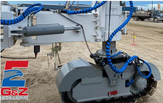
The **SmartLeg** system in tandem with **AccuSteer** allows the swing leg angle to be adjusted on-the-fly to maneuver around an obstacle while automatically keeping the crawler track straight ahead.
