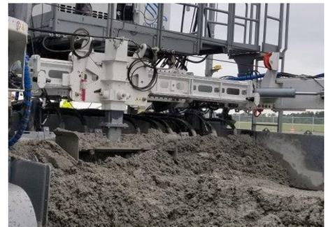
G&Z's powerful and fast concrete spreader plow is easier to change width than an auger. The spreader track sections are tapered pin connected and are light enough to be added / removed by hand with only one retainer bolt per side.
